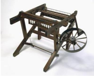
Some say the invention of the Spinning Jenny marked the beginning of the Industrial Revolution: a machine that replaced human beings!
